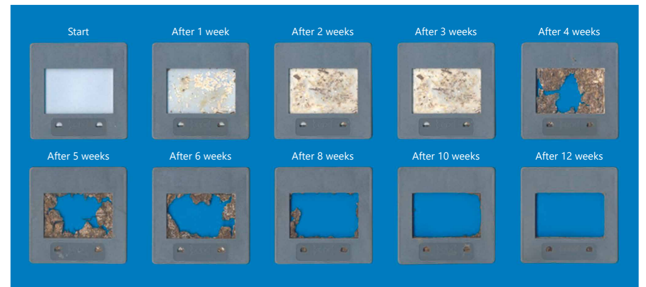
A study published by the "Organic Waste Systems Institute" in Belgium shows that plastic bags made of M-VERA® B5010 with a wall thickness of 288 µm are completely decomposed by bacteria within 12 weeks.
