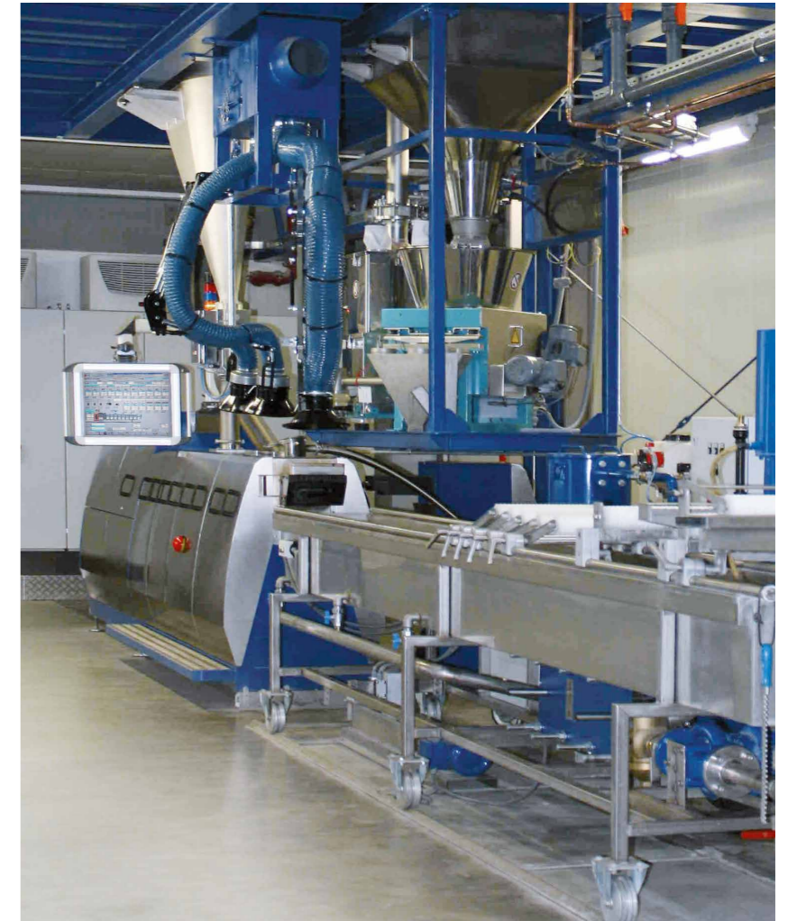
Extrusion line with flexible process length and optional strand or underwater pelletising.
