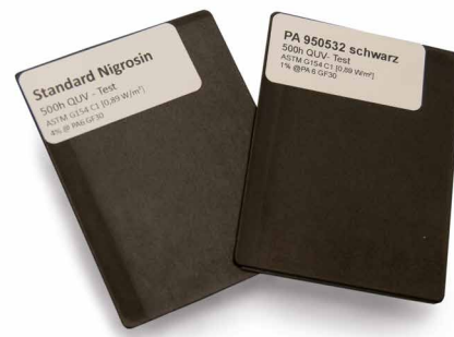
Fig. 3: PA6 GF30 plates, colored with PA 950532 black as compared to a standard nigrosine black according to 500 h QUV tester [ASTM G 154 C1].
