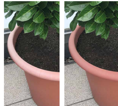
All plastic products are subject to ageing processes. These can be slowed down by the use of additives. The photos show the phenomenon of ageing on a flower pot made of PP (so-called chalking).
