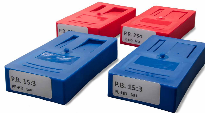
Shrinkage & warpage after recrystallisation can be balanced with our PE-HD nucleating agents.
