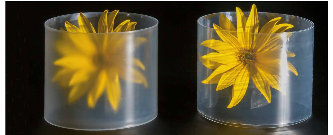
Maximum transparency in PP made possible by the use of clarifier concentrates that are optimised for extrusion or injection moulding processes.
